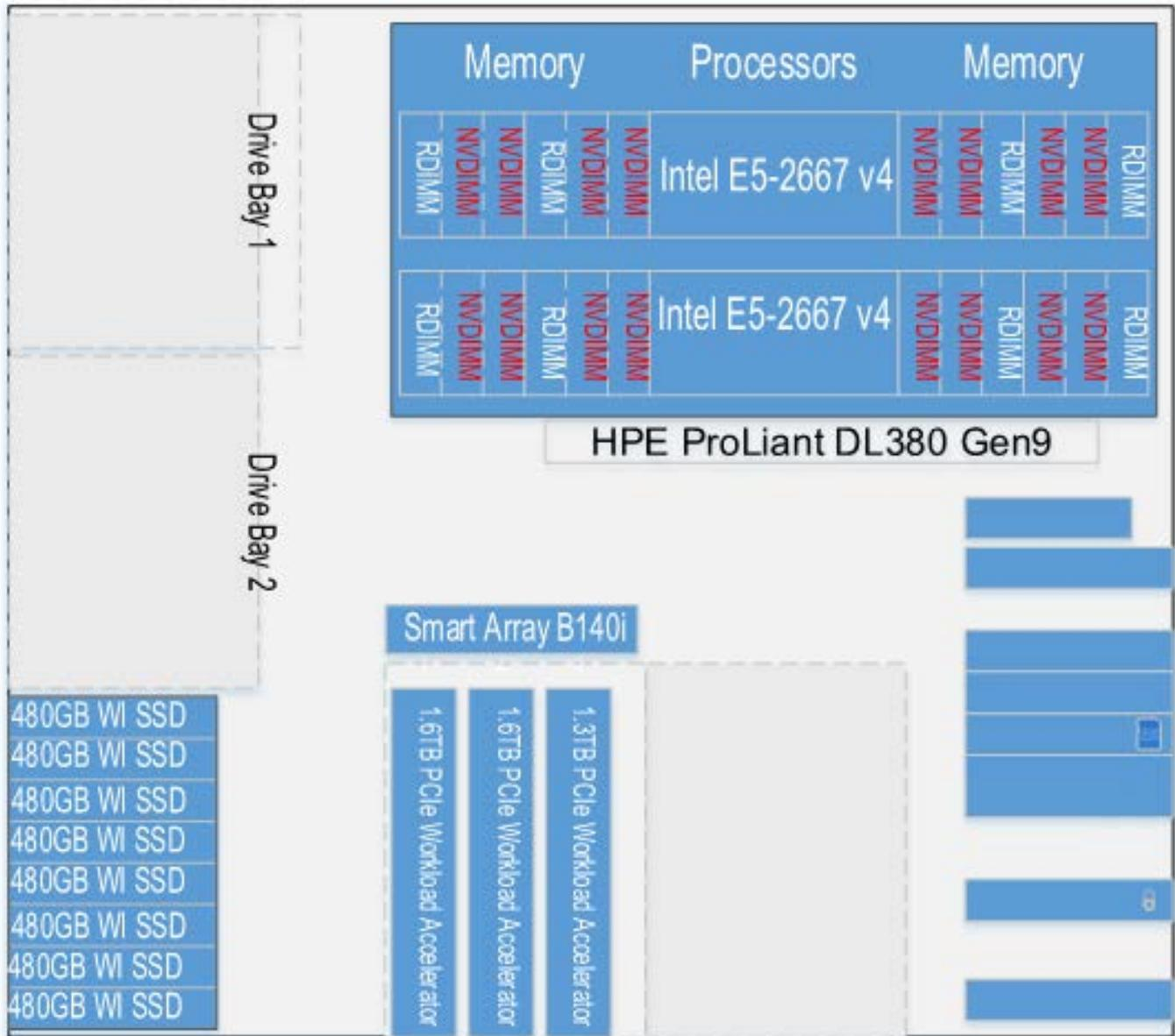
Figure 3. Diagram of memory and disk layout for HPE ProLiant DL380 Gen9 server
